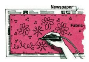
2. Designs may be applied by stamping, line drawing, stenciling, or silk screening.
